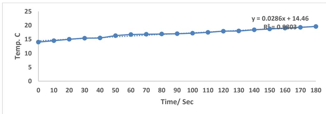
**Figure 2: Calibration of ultrasonic equipment 40 kHz ultrasonic bath, power setting 100%, using 100 ml of distilled water**
