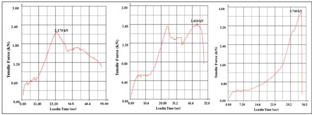
Fig-6: Peel test and final breaking point for "A, B, C" Wood Glue
