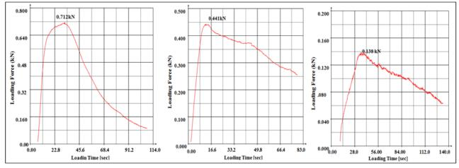
Fig-5: Loading test and final breaking point for "A, B, C" Wood Glue
