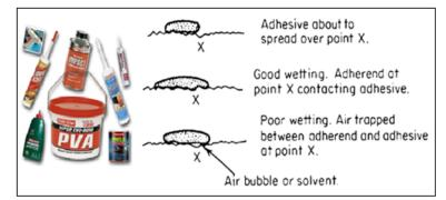
Fig-1: Commercial glue, illustration of good and bad adsorption between Adhesive and Surface
