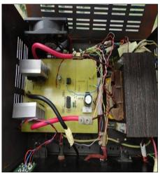
Fig-5: Stage 3 of fixing and soldering components on PCB
