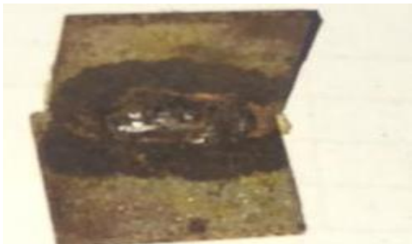
Figure 9: Welded Mild steel Immersion in concentrated HCL with 0.1g/l concentration (AASE inhibitor after 18 hours exposure)
