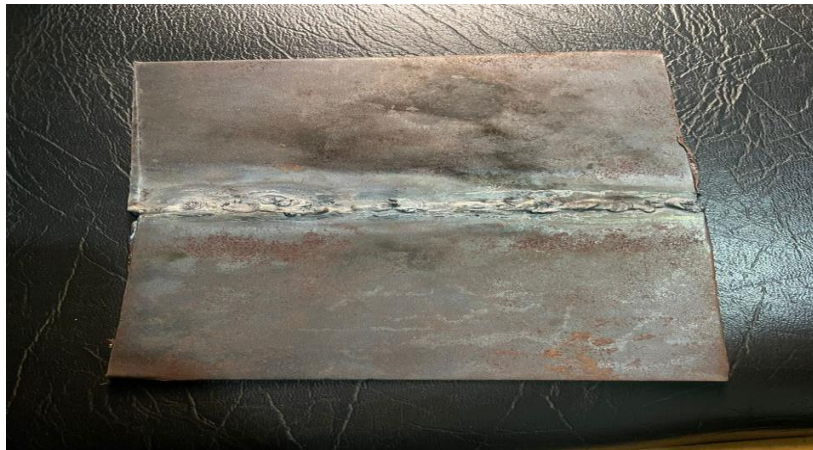
Figure 2: Corrosion Improvement on Welded Mild Steel (Mohammed et al. , 2018)
