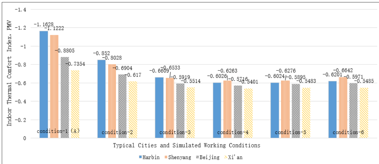
Figure 9: Comparison of PMV values in heating rooms under different operating conditions in typical cities
